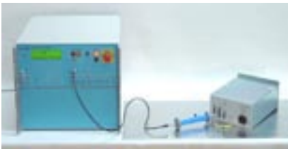
Fig. 2: PIN injection test setup
