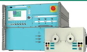
Fully integrated test system for DO-160 section 22 up to level 3. PIN Injection, Cable Bundle. Single Stroke, Multiple Stroke and Multiple Burst. One coupler for WF1, WF2, WF3 and WF5A simplifies the test procedure while reducing setup errors.
